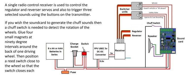
time a magnet passes. The soundcard will then chuff four times per wheel revolution.
