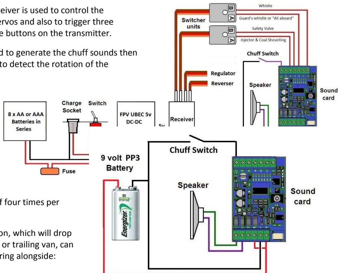
A chuff switch can be set up on the tender or van wheels. The soundcard automatic modes can be used to make a whistle sound on departure and at timed intervals. Other sounds can also occur automatically using the modes provided. A rechargeable PP3 battery should sustain continuous running with an automatic whistle for about two hours.
