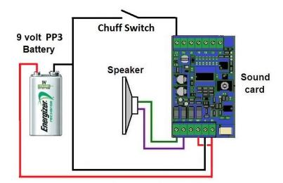
The most common way of doing a chuff switch is to use a reed switch positioned close to the back of a tender or van wheel and then glue magnets around the back of the wheel as follows:
