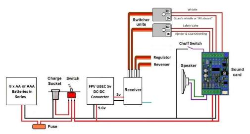
A simple sound installation, which will drop into a locomotive tender or trailing van, can be achieved using the wiring alongside:
