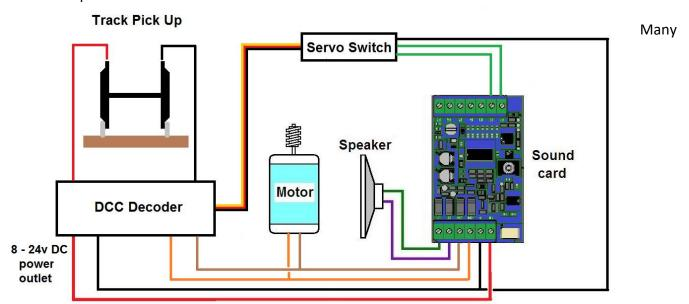
decoders also have function outputs which can be used to trigger sounds. However, this is technically difficult and you should only attempt it if you are very familiar with your decoder and the setting of CVs.
