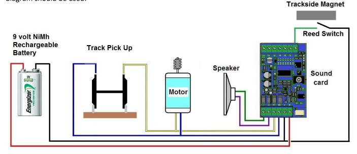
The wiring diagram below shows the connections for the DC jumper board in a Bachmann locomotive.
