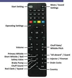
Note that the buttons on the remote control auto-repeat if held down. If you want a single event to occur, like turning on the safety valve, then press the safety valve and release it immediately. If you want to make a large change in volume or tone then you can hold the button down to avoid the need to press the button repeatedly.
