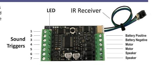
on the left trigger the various sounds where the locomotive controller has the appropriate outputs available. The trigger terminals are labelled F1 to F7 and are referred to by these labels in these instructions e.g. "Triggering F1" means to close a contact between the F1 terminal and the Battery negative terminal.
