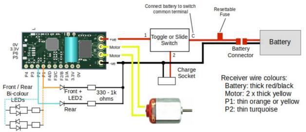
LEDs on P pads should be connected between the pad and battery negative (0V) with a series resistor appropriate to the required brightness.
