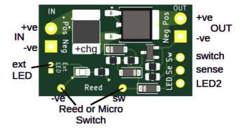
MSW13a is available as: a bare board with or without reed switch mounted; and with optional input, output and charge connector wires. Although there is no solder pad on the board, a positive charge lead may be soldered to the bottom of the fuse so that this is in circuit for charging.
